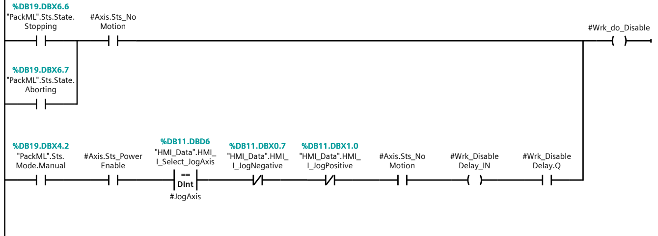
Network 5: Disable delay timer for manual mode - if no jogging for 2 min, disable axis
