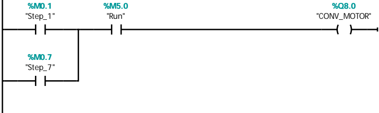
Network 14: Glue sprayer control, on to spray glue
