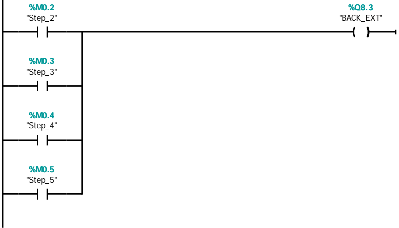
Network 17: Right flap ram extend direction control, on to extend ram
