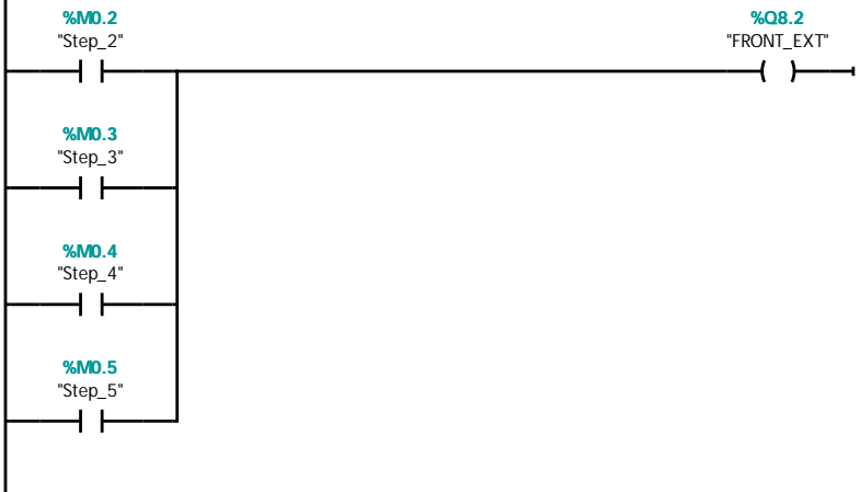
Network 16: Back flap ram extend direction control, on to extend ram
